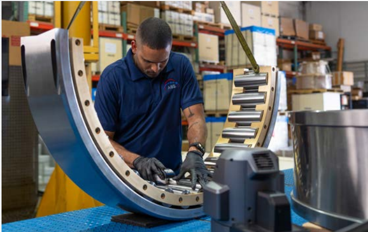
↑ Assembly, quality control and measurement of STRB and the SRB at our Miami operations facility. ↑
