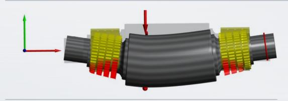
Mill Roll deflection under normal operation conditions generates uneven load concentration between the four roller rows and in each roller itself.
