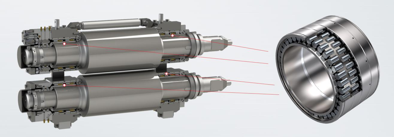
Roll neck bearings are subjected to heavy loads and high specific pressure. The available mounting space is very limited, especially in the radial direction. Consequently, a bearing with a low sectional height but high load-carrying capacity is required.
