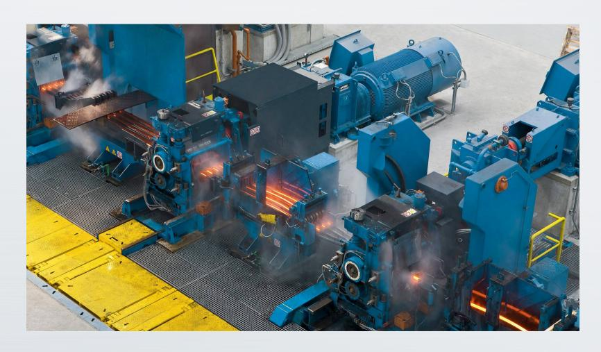
Long-product steel rolling mills are specialized facilities for producing long steel products such as bars, rods, angles, beams, and channels. These mills play a crucial role in steel manufacturing, transforming raw steel into finished products used in construction, infrastructure, and various industrial applications.
