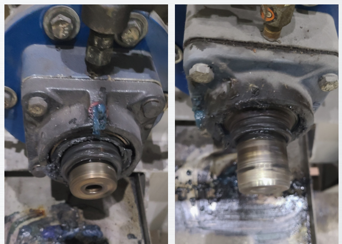
Original design standard 4 bolt flange bearing with the shaft protruding at different lengths because of the different operating parameters.
