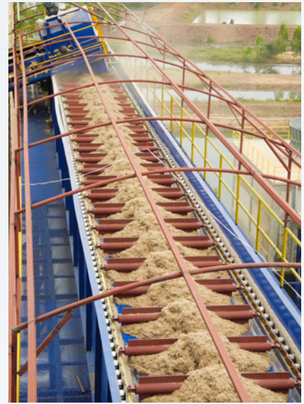
Figure 2-12. Drag conveyor carrying bagasse
