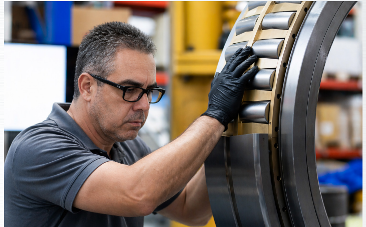
↑ Assembly, quality control and measurement of STRB and the SRB at our Miami operations facility. ↑
