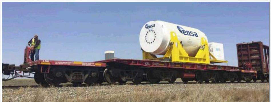
Figure 7. The tested ENUN 32P cask on a rail car in the United States
