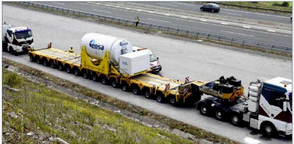
Figure 6. Truck heavy haul in Spain of ENUN 32P cask
