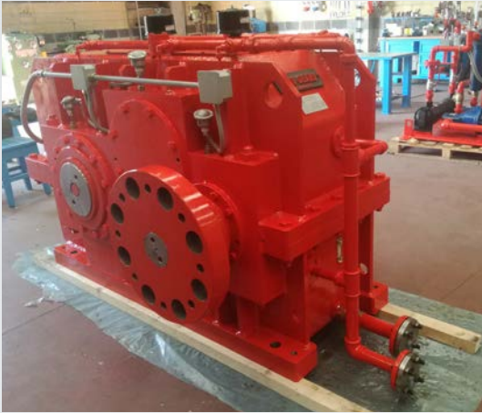
Repowered reducer, equipped with injection lubrication system, monitoring elements, and the included flexible couplings and lubrication system.
