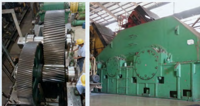
Split torque gearbox repair/upgrade Cement Mill Drive, Italy
