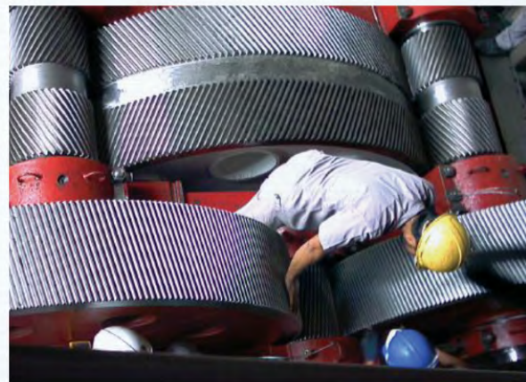
New gear set for a 150 tons split torque gearbox / Cement Mill Drive Tailand
