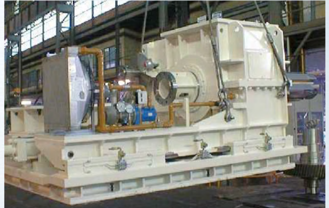
Hot Steel Mill Special Gearbox.Thyssen 35 Tons
