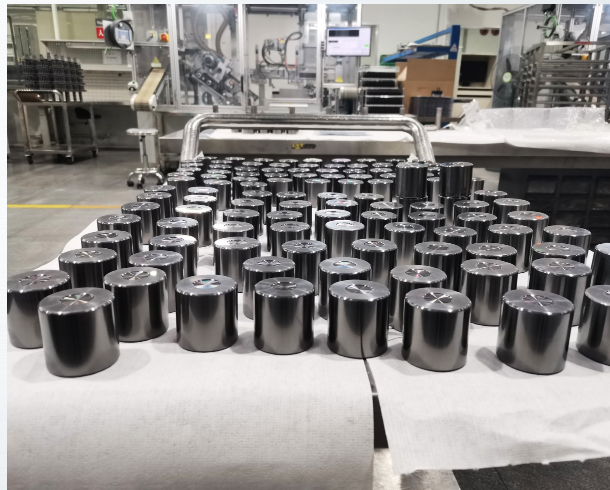
Cylindrical Roller after Triboslide treatment
