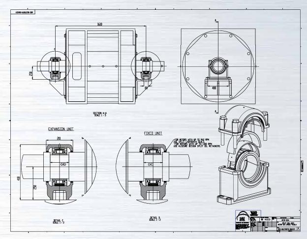
Ex. 5000 HP Synchronic Motor Bearings. Replacing original plain bearing pedestals for triple ring cylindrical roller bearing units.
